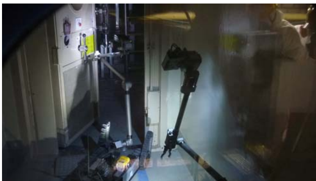
Radio-controlled robot opening the second door of the Unit 3 reactor building at the Fukushima Daiichi NPS (April 17, photo provided by TEPCO)
